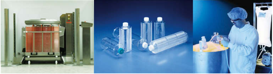
Figure 6.1.9: Disposable systems for the cultivation of animal cells: cell factory, roller bottle, single-use bioreactor (example from Thermo Fisher Scientific).
